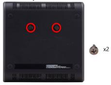
4. Position the Chromebox onto holes on the VESA mount and then push it right to fix the Chromebox. The Chromebox and mount must be vertical.
