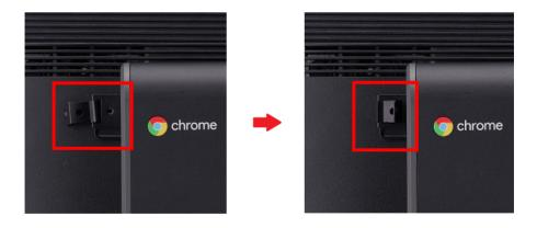
6. Tighten the VESA lock bracket and VESA bracket with provided hexagon screws or phillips screws depending on package contents.
